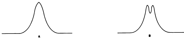
Figure 16. Resonance line emission of a hollow cathode lamp (A) Normal emission. (B) Self-reversed emission, caused by excessive current, or flaws in design
